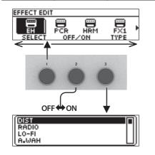
In the CTL & ASSIGN screen (p. 13), WRITE UTILITY screen (p. 15), and MENU screen (p. 16), you can move the cursor and select an icon by operating any knob.
