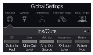
3. Turn the Upper Knob to select one of the submenus. If necessary, press PAGE ▷ to view more parameters.
