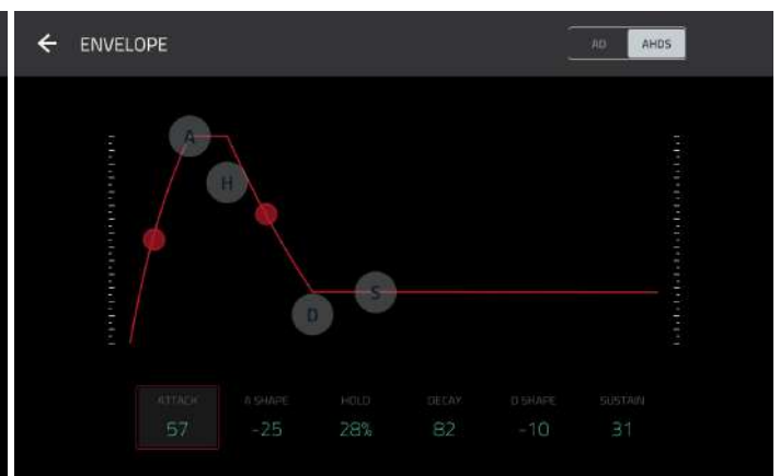
Close-up of an AHDS-type amp envelope.
