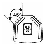
The rear side inclination, symmetrical, as shown in the upper picture, is 45°. SYA12 can be used as a stage monitor in small contexts, in this case please consider the characteristic dispersion pattern presented above.
