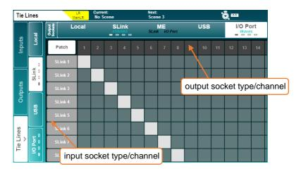
Tie lines are used to patch connections directly between source and destination points without using any of the channel processing, mixing or level control in the core.
