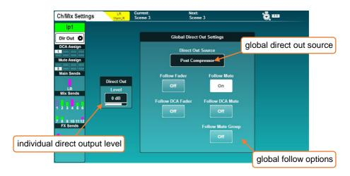
Touch the 'Dir Out' button on any input channel.
