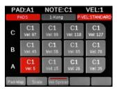
To change the velocity level for a pad, simply select it by tapping the pad and use the Data encoder (O) to change the value.
