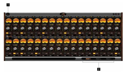
The MP32 software control panel allows you to control all the functionality of its hardware. There are two different types of preamp section on the MP32 control panel, one which is HiZ enabled to the first four preamps and the rest of the preamps which control only mic/line levels.
