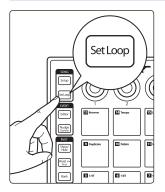
Pressing the Set Loop button allows you to set the start and end points of a timeline loop as well as position it within your session and focus on the loop area to quickly zoom in to make edits.
