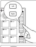
While Set Loop is active, use the right and left buttons to move forward and backward on the timeline.
