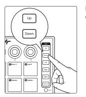
Pressing Zoom with either the Up or Down buttons simultaneously will zoom in or out respectively.
