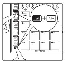
Press Shift and Editor simultaneously to completely close the Pattern Editor.
