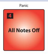
To disable all MIDI signals, press Pad 4 while holding the Setup button.
