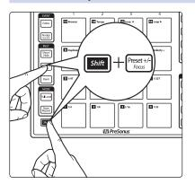
To change the currently focused pad in Impact, press the Shift and Preset +/- button.
