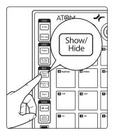
By default, the 16 pads on your ATOM send Note On/Off messages on every bank. Using Advanced Setup mode, you can configure any of the pads on Bank 1 to only send CC messages. To disable Note On/Off for any pad, press the Show/Hide button while Advanced Setup Mode is active. Pads that are illuminated have Note On/Off enabled. Pads that are not illuminated will send CC messages only.
