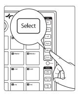
Pressing Select button will create a track and instantiate the currently selected preset, or plug-in if no preset is selected, and bring it into focus for instantaneous control.
