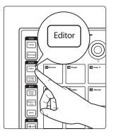
By default, the 22 button functions listed in *Section 5.3* send their MIDI messages on MIDI Channel 1. Pressing the Editor button while Advanced Setup Mode is active will allow you to change the MIDI channel for the buttons on your ATOM.
