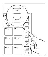
Pressing Zoom with either the Left or Right buttons simultaneously will zoom in or out respectively.
