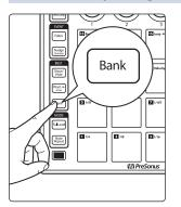
To adjust the brightness of the LEDs on your ATOM, press the Bank button while Advanced Setup mode is active. This will allows you to advance through the three brightness options available.
