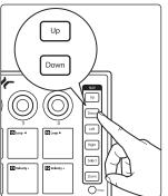
Use the Up and Down buttons to raise or lower the pitch by one half-step.
