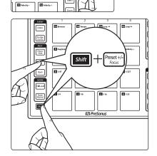
For faster control, enable Pad Focus mode by pressing the Shift and Preset +/- buttons simultaneously while Pattern Editor control is inactive. This will let you audition each pad's sound. Press Editor again to enable Pattern Editor control. This will automatically select the last pad touched.
