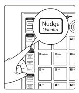
By default, the 16 pads send their MIDI Pressure messages on MIDI Channel 10. Pressing the Nudge button while Advanced Setup Mode is active will allow you to change the MIDI channel on which the 16 pads will send Pressure messages.
