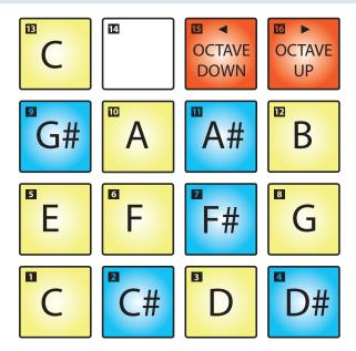
While MIDI Keyboard Mode is active, your ATOM pads will function as a single octave keyboard from C to C in each octave. Pads 15 and 16 adjust the octave down or up respectively.
