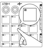
Press the pad assigned to the sound on which you'd like to enable Note Repeat.
