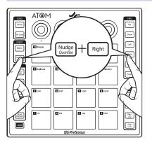
Holding the Nudge button while pressing the Right button, moves the selected event or note forward in the timeline according to the current grid settings.
