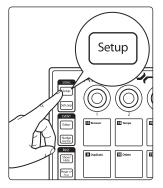
By default, the 16 pads send their MIDI messages on MIDI Channel 10. Pressing the Song Setup button while Advanced Setup Mode is active will allow you to change the MIDI channel for the 16 pads on your ATOM.
