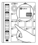
To insert a Pattern part for the current track, press Pad 9 (Duplicate). *For more information on Pattern Editor control, see Section 3.5*.
