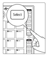
To change the sound that is being triggered, press the Select button and then press the desired pad.
