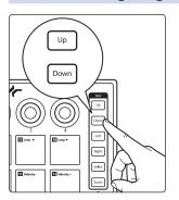
Press the Up and Down buttons to navigate through the track list.
