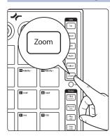
While holding the Zoom button, the Navigation buttons allow you to adjust the current view.
