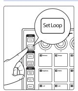
By default, the 4 knobs send their MIDI messages on MIDI Channel 1. Pressing the Set Loop button while Advanced Setup Mode is active will allow you to change the MIDI channel for the 4 knobs on your ATOM.
