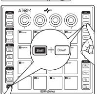
Press the Shift button with the Up or Down buttons to change the pitch by an octave.
