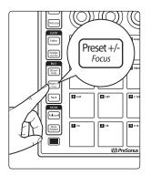
When the Instrument plug-in window is open, you can quickly change presets by pressing Preset +/- button. Press and hold for momentary. Press and release to latch.
