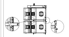
6) Reverse and connect the rear bracket of the second cabinet using the hole.
