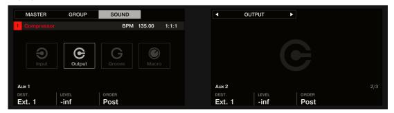
7. Use Knob 2 (Aux 1 LEVEL) to adjust the level of the signal sent to that auxiliary output.
