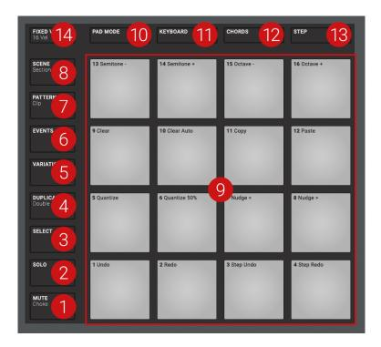
The Pad section: the Mode buttons (1) to (8), the pads (9), and the Pad Input Mode buttons (10) to (14)
