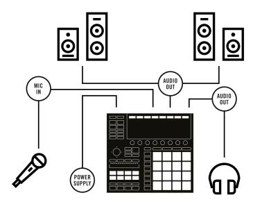
MASCHINE+ setup with a dynamic microphone.
