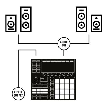
MASCHINE+ setup with active monitors.
