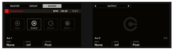
6. Turn Knob 1 (Aux 1 DEST.) to assign the first auxiliary output to the desired send effect. In addition to the usual entries available in both fields, you will find all the Sounds and Groups with an Effect Plug-in loaded in their first Plug-in slot — see Step 1: Set Up a Sound or Group as Send Effect For each Sound, the entry shows the Group letter and number followed by the Sound number (in the example underneath we selected the entry A1:S1-1 for the Aux 1 output).
