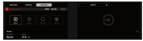
You will now see two parameters at the bottom of the left display: **SOURCE** (which selects the source) and **GAIN** (which adjusts the level of the input).
