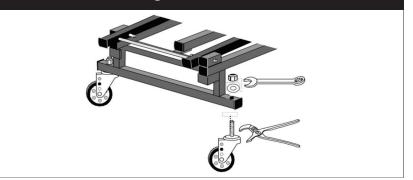
Attach front swivel casters as shown. While tightening lock nuts, grip bearing cap with channel lock pliers or pipe wrench to prevent threaded stem from turning. Tighten lock nuts firmly, but not excessively tight. Check lock nut tightness on caster stems periodically.
