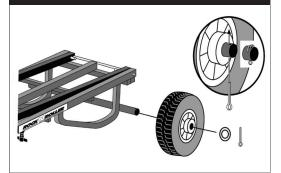
Gently slide wheel over axle as shown. Do not force wheels onto axle. It is recommended to lubricate axles with light grease before installing. Install cotter pins and bend ends outward.
