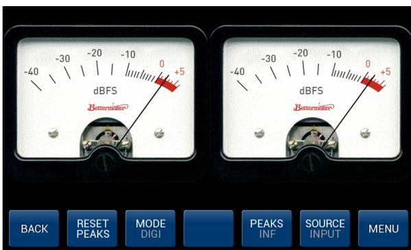
VU – Volume Unit Meter, calibrated to show 0dB when 0dBFS 1kHz sine signal is present. The fall time is the same as the integration time - 300 ms.
