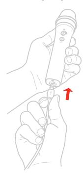
2. Connect the Lightning cable to the connector on your iOS device.
