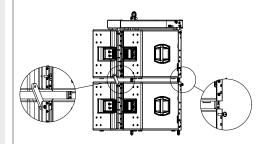
6) Reverse and connect the rear bracket of the second cabinet using the hole.
