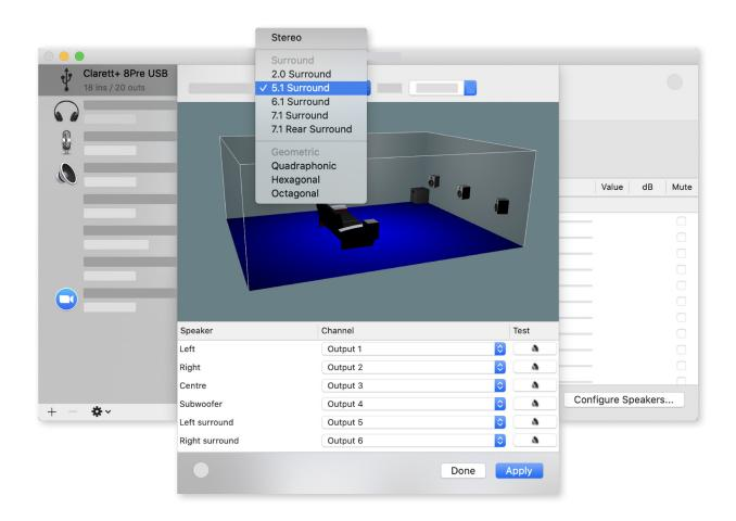
The example below shows how you would connect the six loudspeakers in a 5.1 surround monitoring arrangement
