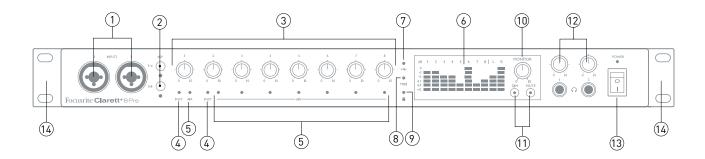
The front panel includes all input gain and monitoring controls as well as two input connectors for Mic, Line and Instrument signals.
