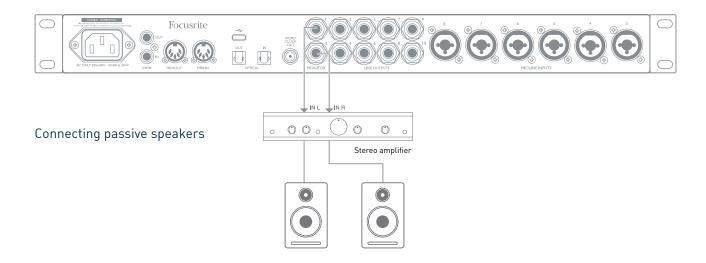
All the line output connectors are 3-pole (TRS)  $\frac{1}{4}$ " jack sockets, and are electronically balanced. Typical consumer (hi-fi) amplifiers and small powered monitors will have unbalanced inputs, either on phono (RCA) sockets, or via a 3.5 mm 3-pole jack plug intended for direct connection to a computer. In either case, use a suitable connecting cable with jack plugs at one end.
