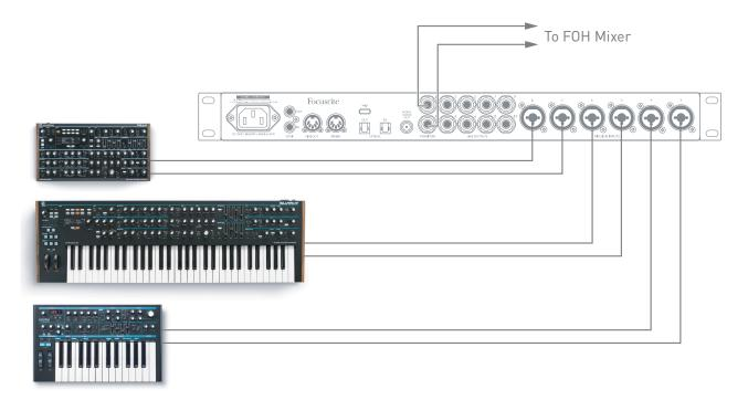
In the example illustrated, three stereo keyboards are connected to rear panel inputs of the Clarett+8Pre; Outputs 1 and 2 connect to the main PA system. You can adjust the volume of the individual keyboards from the front panel, and you can adjust the level you hear the mixed keyboards at through the speakers.
