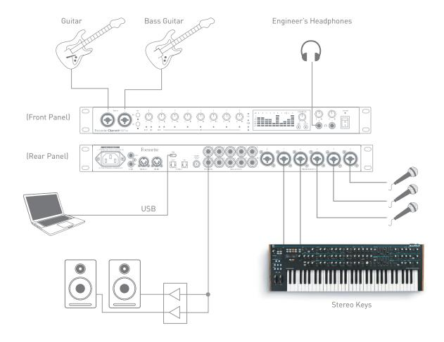
This setup illustrates a typical configuration for multitrack recording with DAW software on your computer.
