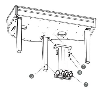
4. Put the pedal assembly line on the plug body pedal jack.
