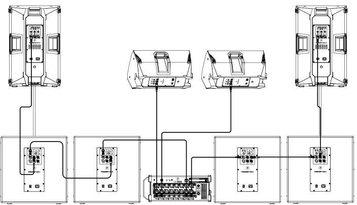
Here's how to set up a large club system. In this example, the L/R outputs of a DL16S mixer are connected directly to the channel A inputs of a pair of Thump118S subwoofers. The Full Range Out of each subwoofer is then connected to the inputs of an additional pair of Thump118S subwoofers.
