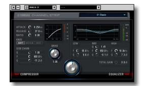
**Sweet Spot Morphing Channel Strip:** a sidechain-enabled compressor and a 3-band parametric equalizer.
