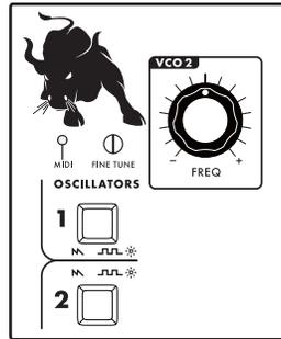
The Oscillators are the main sound source of the Minitaur. They create electronic vibrations that can be tuned and amplified into sound that we can hear. The Minitaur's VCOs can produce a total musical range of 6 octaves.
