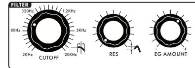
The FILTER is a classic Moog 24dB/Octave Low-Pass Filter design with resonance. It has controls for CUTOFF frequency which determines the range of frequencies the filter will affect, as
