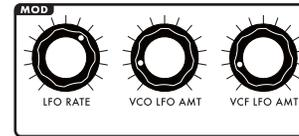
MODULATION is an important part in the creation of musically-expressive sounds. The Minitaur's MODULATION section provides an LFO with adjustable RATE and AMOUNT controls for the oscillators (VCO) and the Filter (VCF). The Low Frequency
