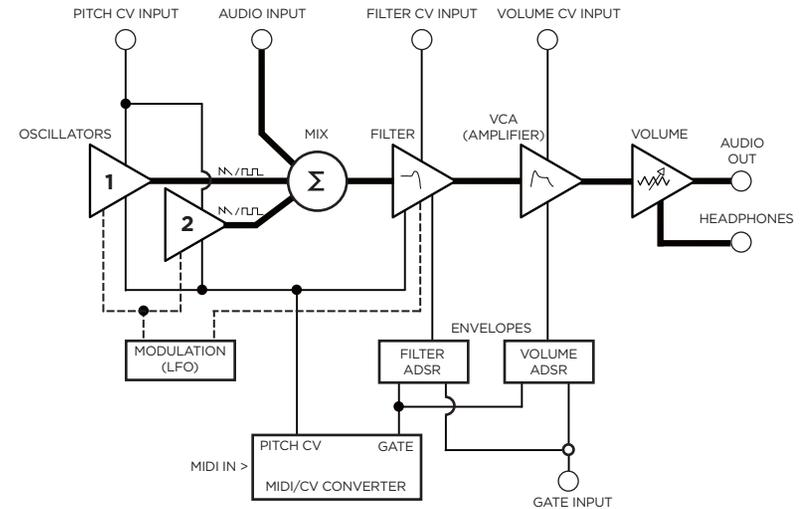
The Minitaur's source signals are created by two Voltage-Controlled Oscillators (VCO) which are mixed with the External Audio Input. The Mixer Output is routed to the Filter, where the tone is sculpted according to the Filter parameters and the Filter ADSR Envelope. The signal is then passed to the Amplifier (VCA) stage, where the Volume ADSR envelope shapes it. Finally, the signal is routed to the Output section, where the final level is set by the Volume control knob.
