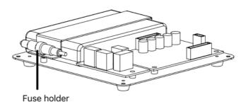
In case fuse is blown, you need to replace it. Unplug the fixture from power, remove the 4 screw from the housing to find the fuse holder. Open the fuse holder by turning it anticlockwise; remove the blown fuse from the holder and replace it with the exact same type and rating one. Close the fuse holder by turning it clockwise to tighten it. Screw back the base to the housing.
