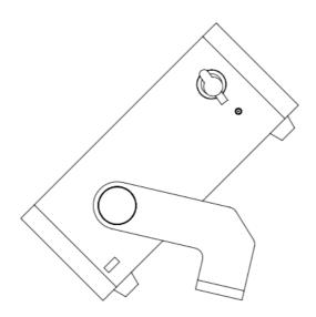
When install the fixture to crossbar and truss, always use an extra safety cord (not supplied with the fixture). Users also need to make sure the crossbar is stable or not moving, and can support a weight of 16 kg (fixture net weight 1.6kg).
