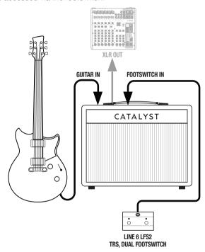
\*NOTE: Optionally, you can connect two individual single footswitches to the FOOTSWITCH jack using a 1/4" TRS splitter adapter. Momentary type footswitches can be assigned to work with your CATALYST via the CATALYST Edit software.
