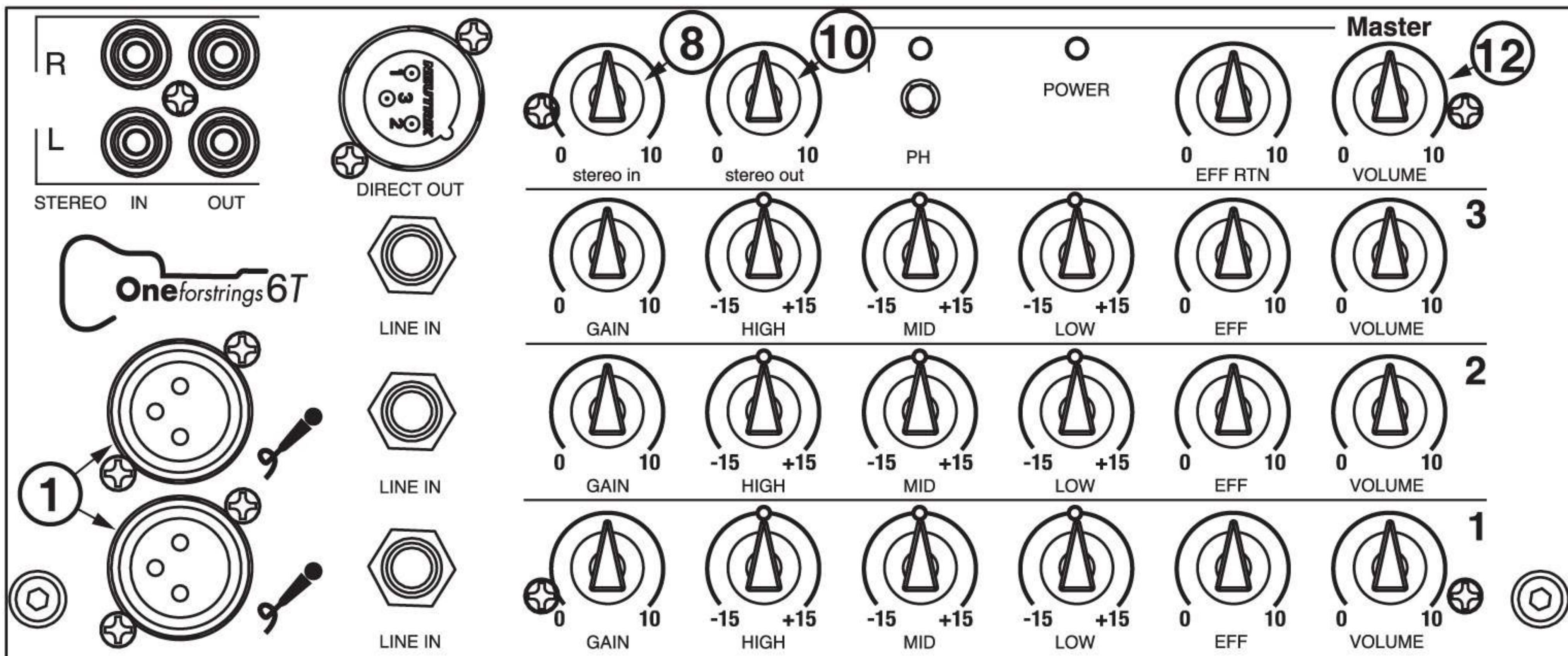
**1-MIC IN:** electronically balanced microphone input with input impedance of  $1\text{K}\Omega$ , input suitable for all types of microphones.
