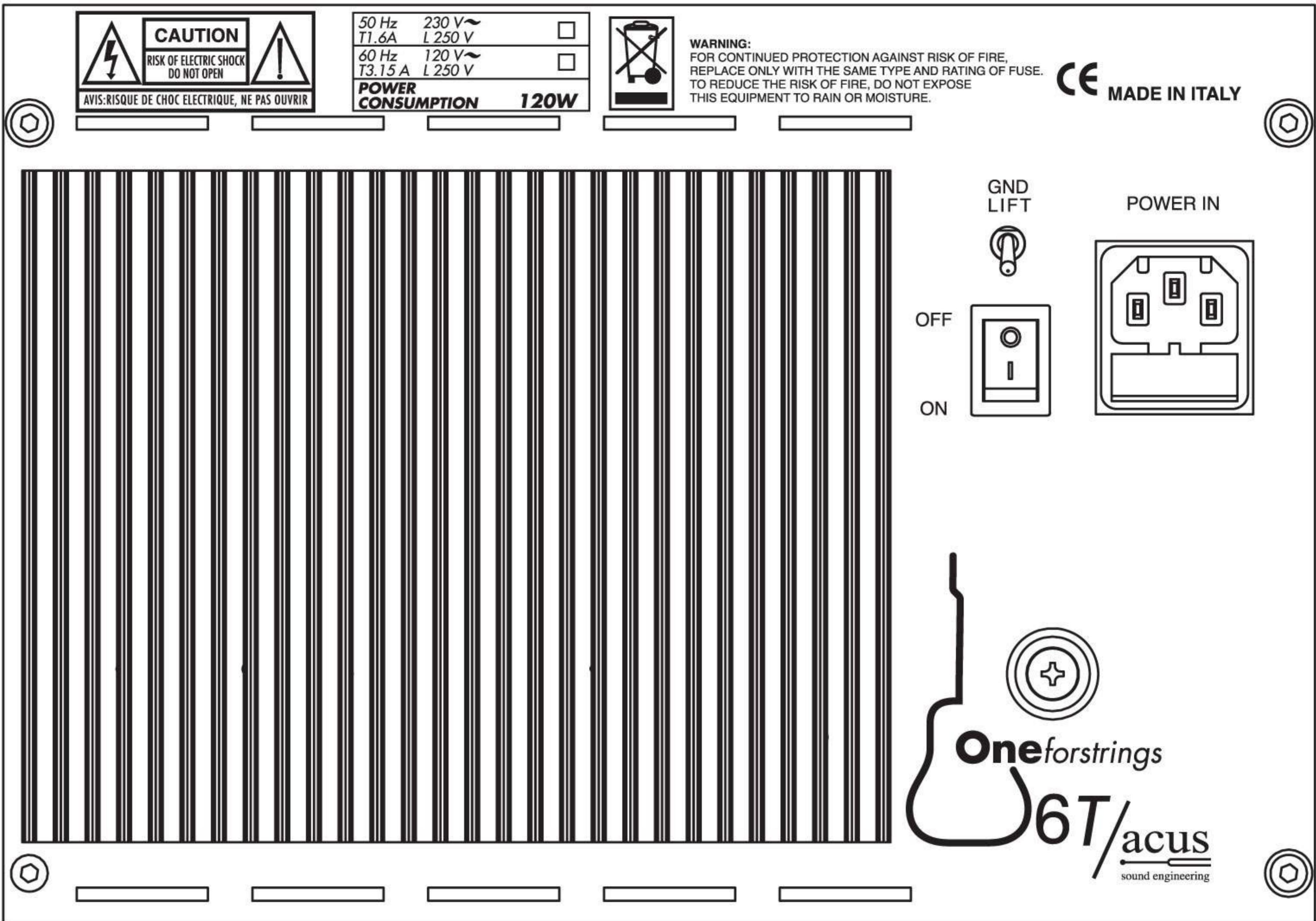
**16- GND LIFT:** switch for grounding the electrical circuit. Revert the position in the event of a humming noise generated by the power supply.
