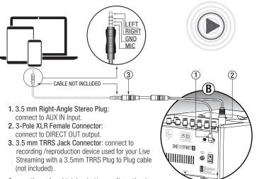
Suggestions: for obtaining better configuration is very important to have a moderate volume to the amplifier DIRECT OUT output. If the amplifier is equipped with the attenuation switch (labeled with -10dB) push this switch for a very easy and fast signal level matching.
