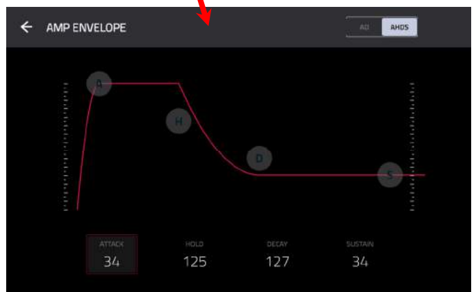
Close-up of an AHDS-type amp envelope.
