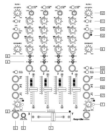
1 VCA Crossfader. The XONE:92 uses eight high performance voltage controlled amplifiers (VCA), a pair for each music channel. The robust 45mm fader produces a DC control voltage which determines the signal level of the VCAs. The voltage is filtered to prevent any audible noise, clicks or scratchiness resulting should the fader track become worn. This benefit would not be possible if the signal were routed through a conventional audio fader.
