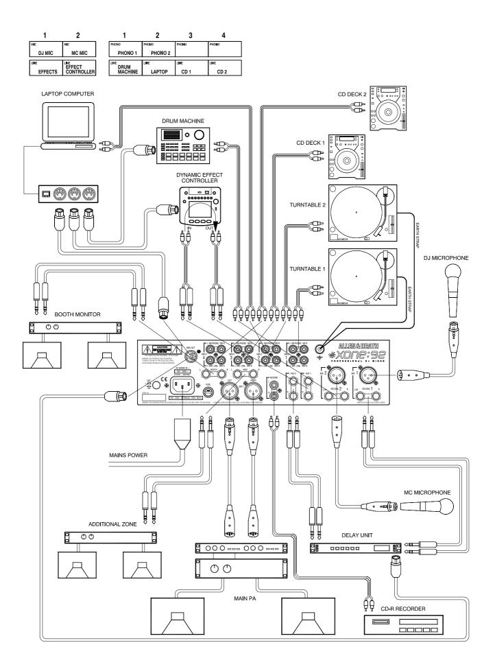
This diagram shows an example hook-up to demonstrate how the **XONE:92** can be connected in a typical DJ application. Note that you do not need to connect the channels in the order shown, also that the connector types on the equipment you connect to may be different to that shown. Use cables appropriate to your application. Please read **Plugging Up The System** before connecting to your equipment. The following describes how the console is used in this example application:
