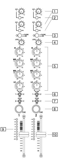
**AUX 1-2 sends**. Adjust the levels of the channel signals to the stereo Aux outputs. Turn fully anticlockwise to turn the signal off, fully clockwise for a maximum +6dB boost.
