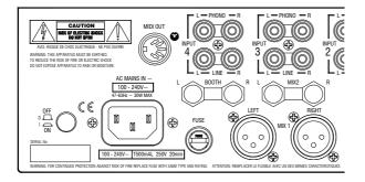
Read the **SAFETY INSTRUCTIONS** printed at the front of this User Guide and on the rear panel. Check that the correct mains lead with moulded plug has been supplied with your console. The power supply accepts mains voltages within the range 100-240V without changing any fuses or settings.
