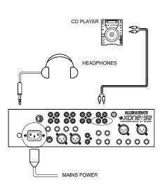
**Set all controls to their starting condition**. Set all FADERS (rotary and linear), LEVEL, AUX, FREQ, RESONANCE, LFO DEPTH, HEADPHONES and BOOTH MONITOR controls to minimum. Set EQ controls to their detented centre position. Set all press switches to their up position. Set all toggle switches to their centre position.
