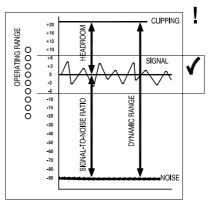
The diagram above illustrates the operating range of the audio signal.
