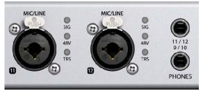
The analog outputs 9 to 12 feed the headphones outputs **Phones 1** and **Phones 2**. These low impedance outputs of highest quality are able to drive headphones at higher levels undistorted, no matter if low or high impedance headphones are used.
