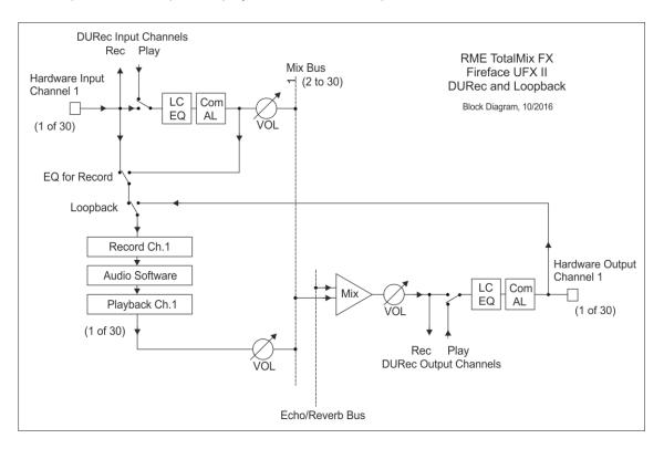
The block diagram shows the signal flow for various situations, depending on the state of *Loopback*, *EQ* for *Record* and *Play active*. In the diagram Loopback and EQ are switched to off, but a playback is active in the input.
