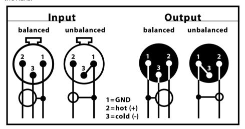
Both output stages operate in parallel, so it is possible to connect two different destination units simultaneously, for example to record to two different media at the same time or split the output between a mixer and effects processor. However, only one type of input (jack or XLR) should be connected at a time – the Auto Dynamic De-Esser is not intended to be used as a mixer!
