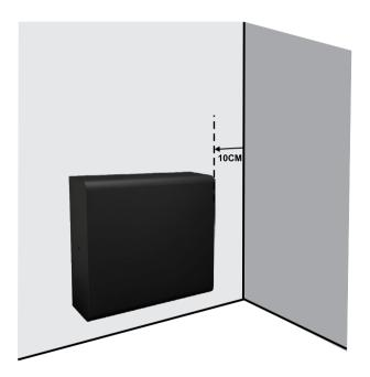
Do not block the bass ports at the side of the loudspeaker. Keep at least 10 cm of free space between the ports and the adjacent wall.
