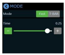
When T-Bar is enabled, all operation could be checked on PST window. Slide T-Bar to switch between PST and PGM.
