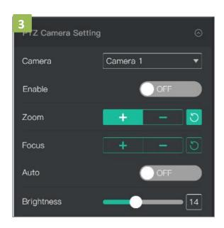
3. After IP address setting, turn on "Enable" and you can control PTZ camera.
