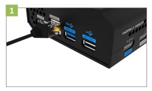
1. Connect the mini-pro to the router's LAN port.
