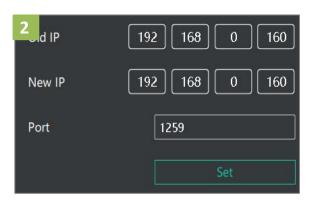
2. Set both old IP and new IP to the camera IP address you want to control,the corresponding communication port to 1259 on mini-pro, configuration path:  $M(Menu) \rightarrow FX \rightarrow PTZ$  Camera Setting Port on the control software of mini-pro.
