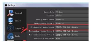
1. Set the audio source: Setting→Audio→Mic/Auxiliary Audio Devices
