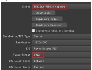
**Note:** If there is no video format YUY 2 after setting above, check the USB 3.0 port connection. Make sure it is linked to USB 3.0 port on PC by USB 3.0 cable. (USB 3.0 cable or port is standard in blue while USB 2.0 is in black). If the captured, change the video format to YUY2.
