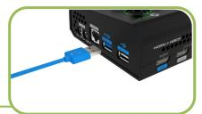
**Note:**If your computer only has a Type-C port, you can use a USB-A to Type-C cable to transmit the webcam signal. Please note that the Type-C cable you choose needs to support data transmission. The signal is recognized in Windows and MAC system as \[ \text{RGBlink USB 3.0 Capture} \] .
