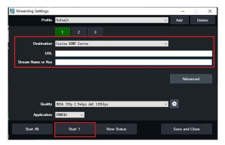
**Note:** vMix does not support automatic recognition of the output resolution of mini-pro. Every time the output resolution of mini-pro is modified, the picture on vMix will pause. The user needs to re-select RGBlink USB3.0 Capture and manually input the current output resolution of mini-pro.
