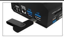
mini-pro will automatically recognize the hard disk or U disk and display the relevant information on the recording window of multi-screen PVW .
