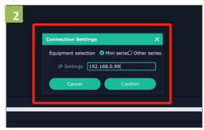
2. Fill in the IP Address of the mini-pro(as example above, default mini-pro IP is 192.168.0.99), and click "Confirm".
