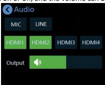
The audio input can be selected as MIC passive microphone input, or LINE input audio console or active microphone signal input according to needs.
