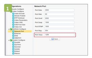
1. Set the corresponding communication port on the PTZ camera, such as VISCA or UDP port 1259.
