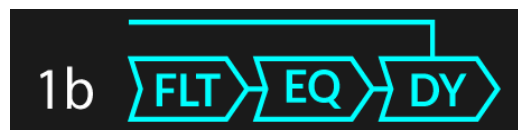
'b' equivalent - the top line going into Dynamics means that the Dynamics sidechain is set to EXTERNAL
